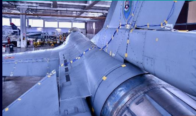
Accelerometers on F16 structure
