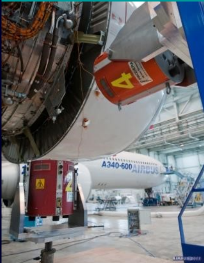
PRODERA shakers on Airbus 340-600 engine
