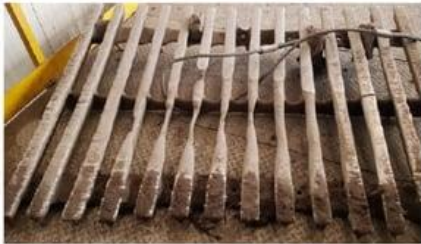
Severe abrasive wear of beams and blinding with a sieved material.
