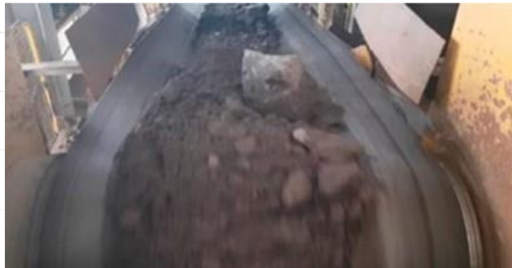
The oversized pieces of material cause failures and create non-Gaussian impulsive noise in signals.
