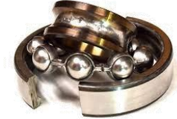
A bearing defect
