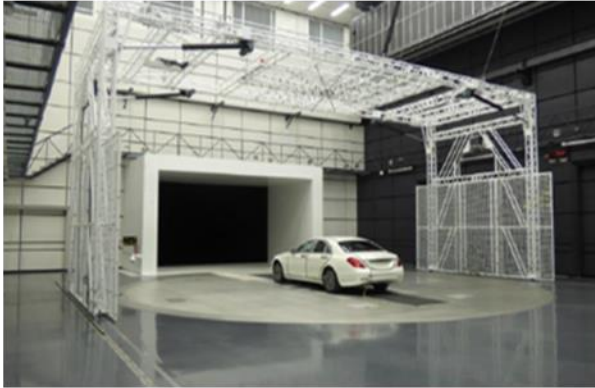
Acoustic measurements in a wind tunnel (typical configurations include a few 100 channels)
